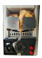
6. Close the tube clamp by turning the cam clockwise, and close the warmer front door.
